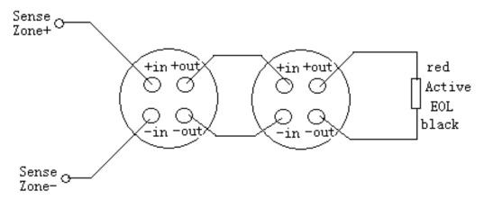
The panel is supplied with 5.1K end of line resistors as standard. Active end of line units are available separately.
