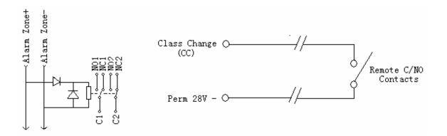
A relay may be connected anywhere on the alarm zone wiring provided that two diodes (1N4001 or equivalent) are fitted as shown in the diagram. The end of line resistor is not shown, but must be connected at the end of the alarm zone wiring. The relay must have a 24V DC coil.
